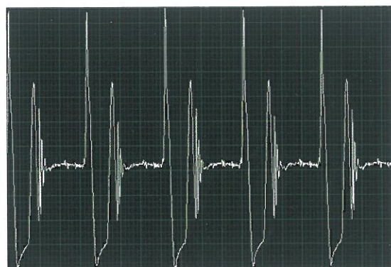
气缸盖零件工作应力测量 Working stress test for cylinder head
