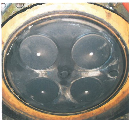
长期燃用重油气缸盖底面情况 Undersurface state of cylinder head of engine longtime operated on HFO
